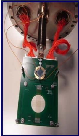
**MCP & grid beam monitor**
