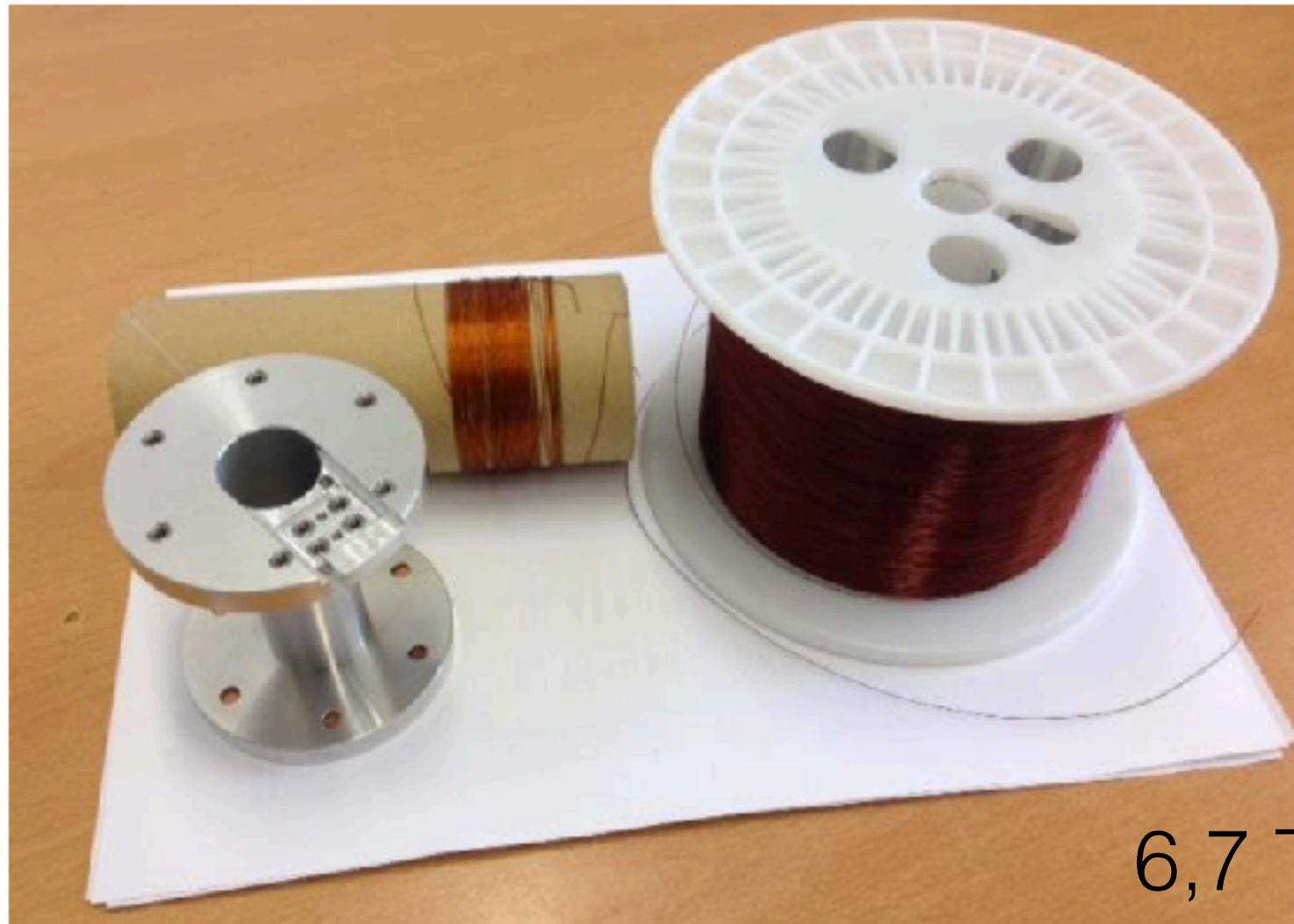
Superconducting Magnet former and superconducting wires
