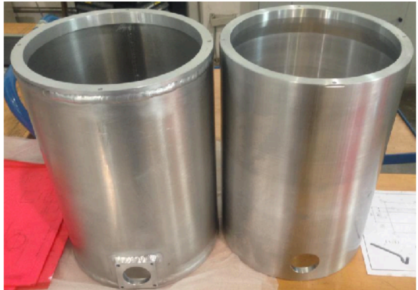
Dewar prototypes manufactured by Payr Production GmbH
