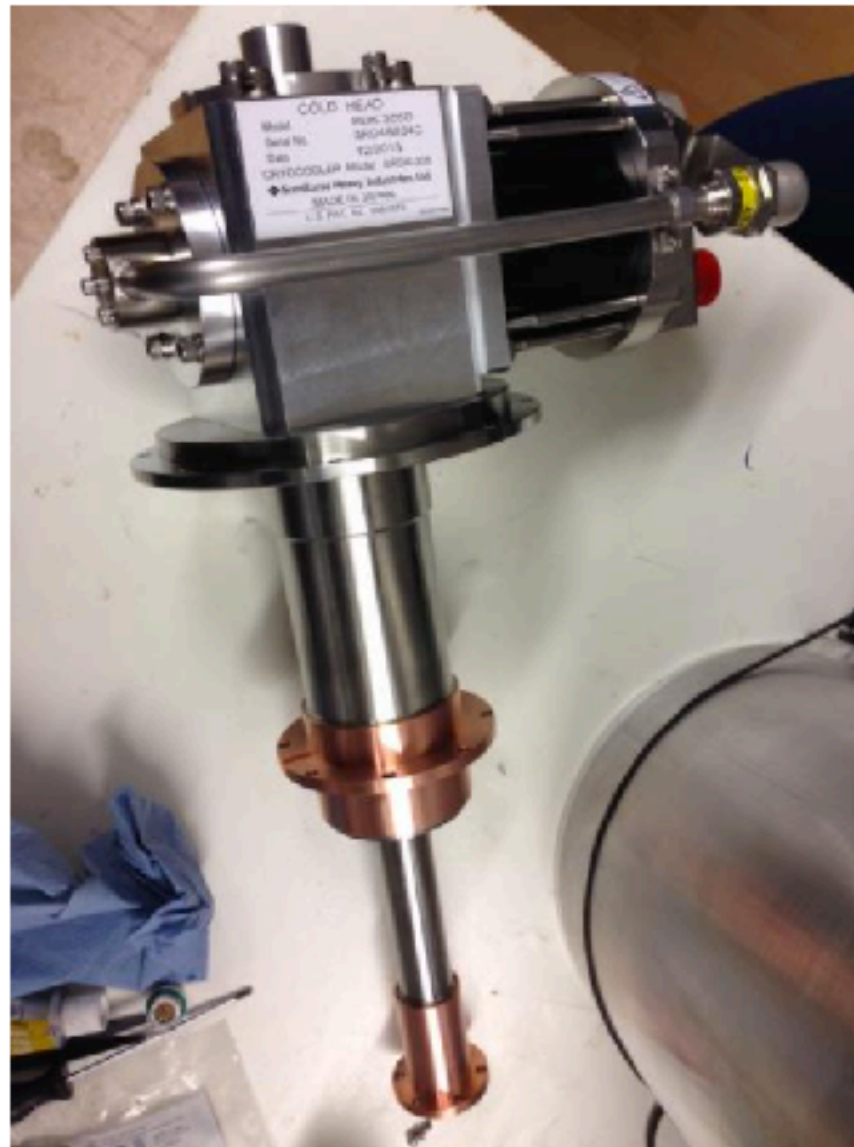
Sumitomo Cold Head and innovative heat-switch prototype
