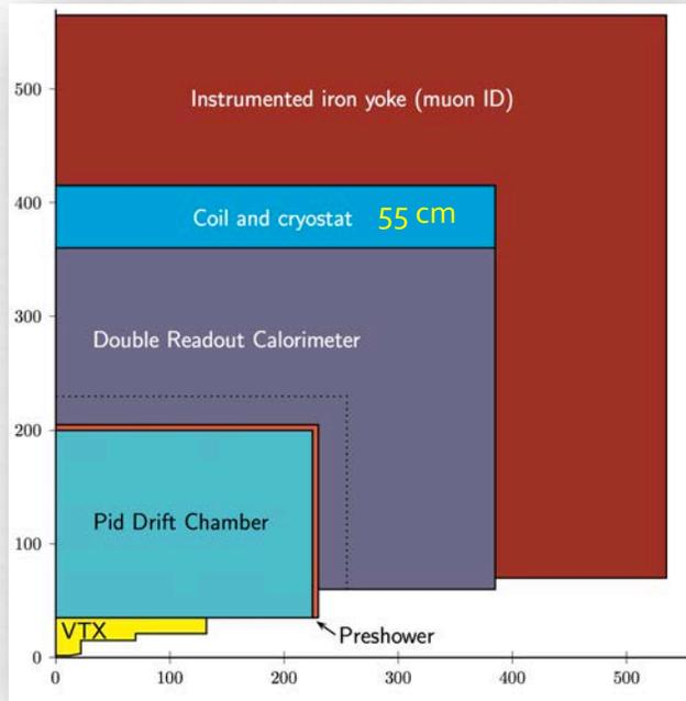
coil inside the calorimeter
