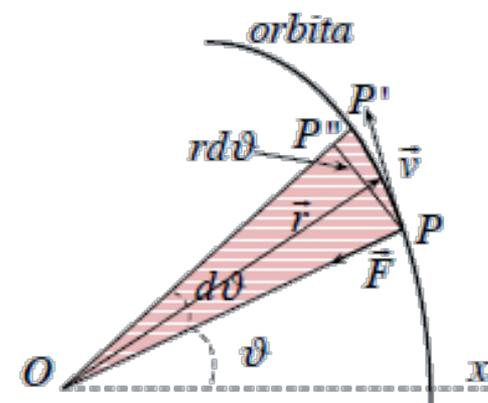
$$\frac{dA}{dt} = \frac{1}{2} r^2 \frac{d\vartheta}{dt} = \text{cost} \quad \text{Per la SECONDA LEGGE DI KEPLERO}$$
