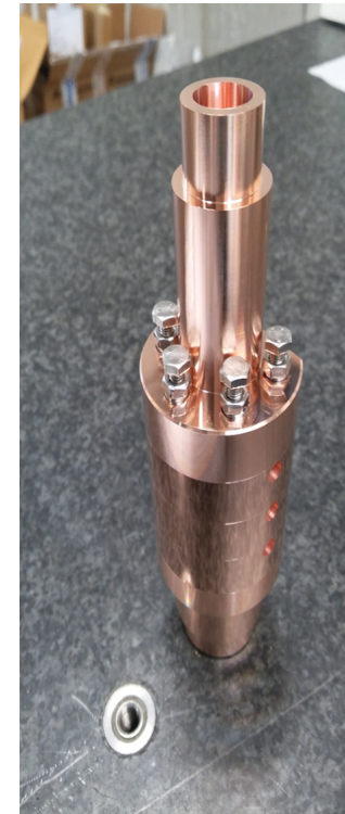
Assembled before welding
