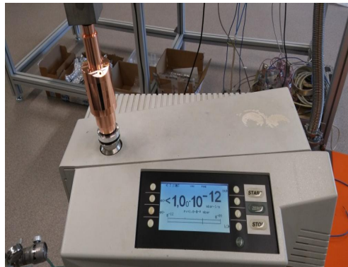
Pre-welding measurements: Excellent vacuum tightness
