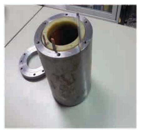
The coil of the primary winding was not designed for the purpose of a good uniformity of the magnetic field because he was designed as pure solenoid with the following radius over length ratio
