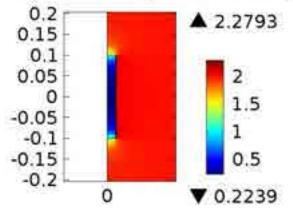
In a cylindric superconducting cavity, even without ending plugs the field inside is fully shielded: FEM with a uniform field 0->2T and  $J_{c0}=2 \ 10^9 \ A/m^2$  and a "Bottura style"  $J_c(B)$ .
