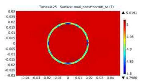
The field lines fully penetrate the cavity inner volume, and the only shielded part is the volume occupied by the superconductor.
