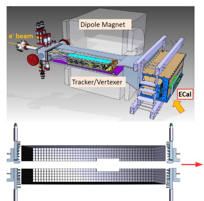
**Design:** PbWO<sub>4</sub> crystals with LA-APD readout
