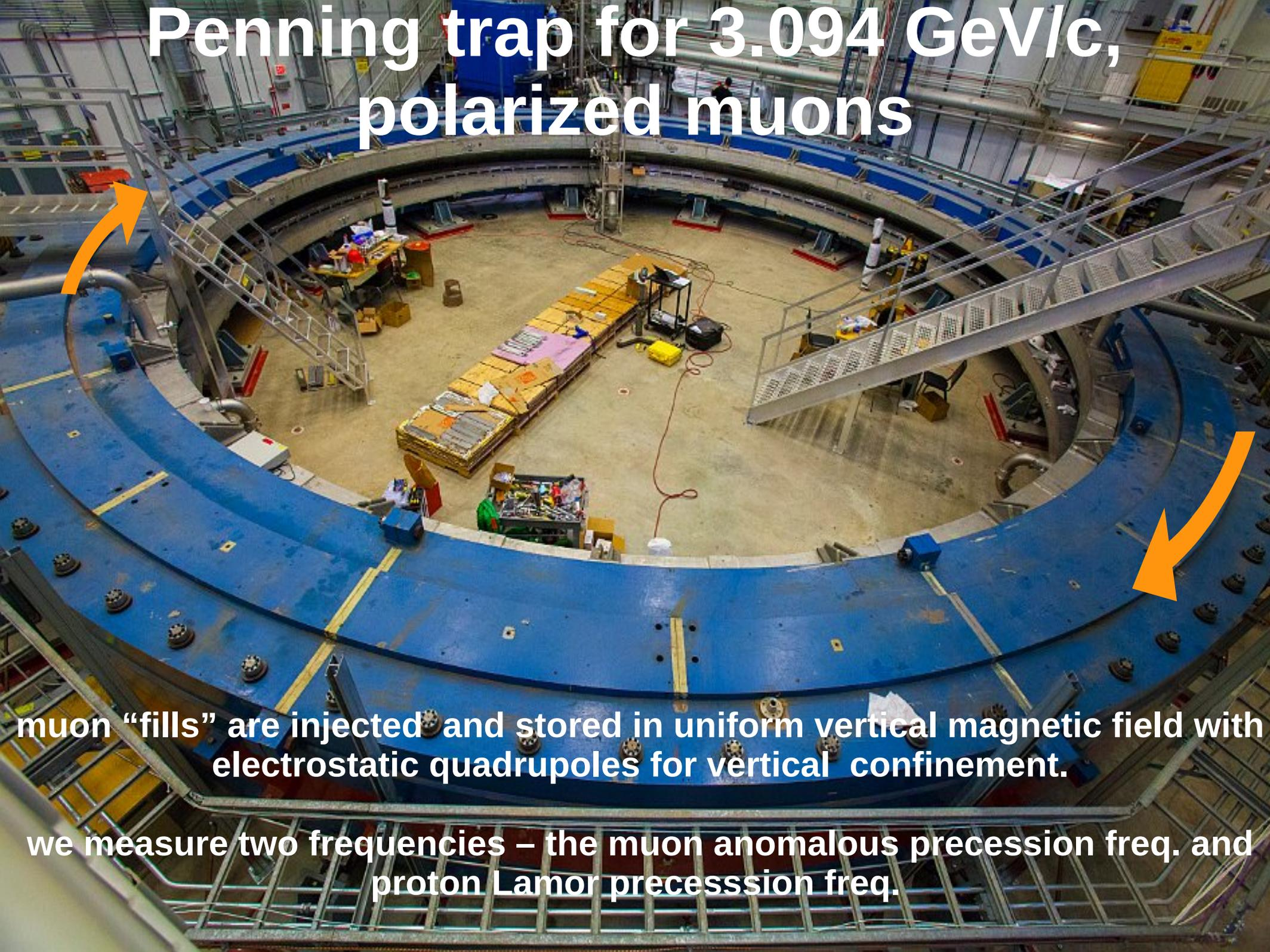
muon "fills" are injected and stored in uniform vertical magnetic field with electrostatic quadrupoles for vertical confinement.
