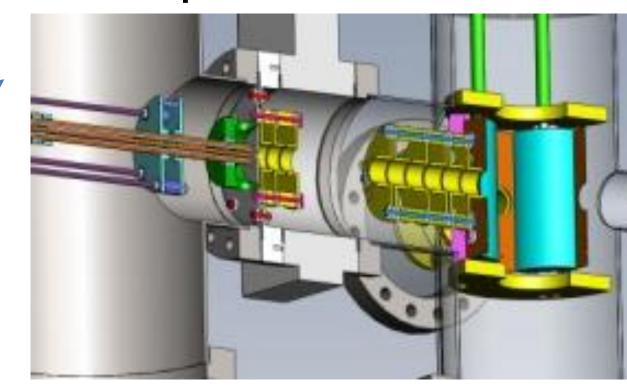
The ion optics (stacks of biased electrostatic lenses) guide the cluster ions through the differentially pumped vacuum system. In order to avoid losses and to increase transmission. The bender consists of four cylindrical plates which are biased to a tunable potential in such a way that the incoming ion beam is subjected to the Lorentz force **F**=q(**E**+**v**×**B**). The particles are thus **deviated** by 90° in order to separate the cations from the neutrals and the anions.
