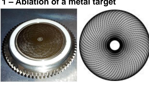
The second harmonic ( $\lambda$ =532 nm) of a high frequency pulsed Nd:YAG laser source is used to ablate the surface of a metal target and to produce a hot metal **ion plasma**.
