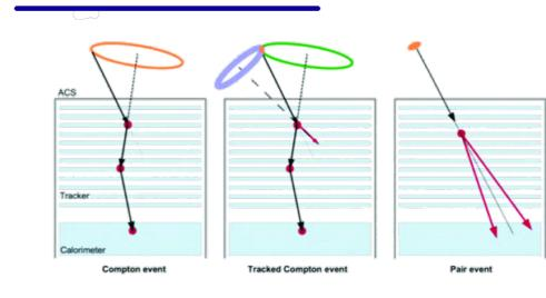
Like other gamma ray telscopes, eAstrogam consist of three main detectors: a Tracker made of several SI thin layers of double sided strip detectors (DSSD), a **Electromagnetic Calorimeter** made of an array of CsI scintillation crystals and a **Anticoincidence System** realized with plastic scintillators.
