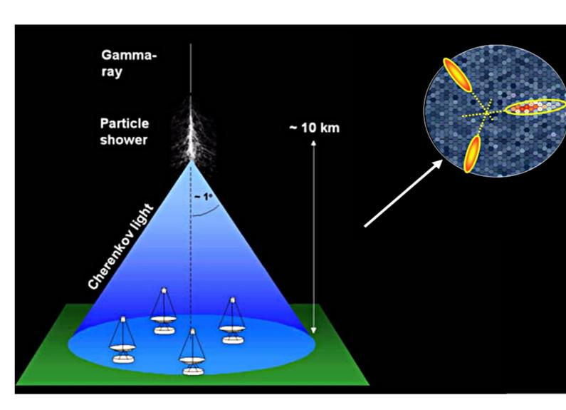
The detection of gamma rays using Imaging Atmospheric Cherenkov Telescopes (IACTs) is possible thanks to the Cherenkov effect: the incoming gamma-ray, interacting with the atmosphere, produces an electromagnetic shower. These particles travel faster than light in air, and so emit a characteristic blue light (up to the UV band), called Cherenkov radiation.
