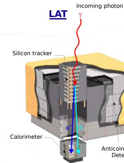
The Large Area Telescope (LAT) is designed to detect gamma rays via the pair production mechanism.
