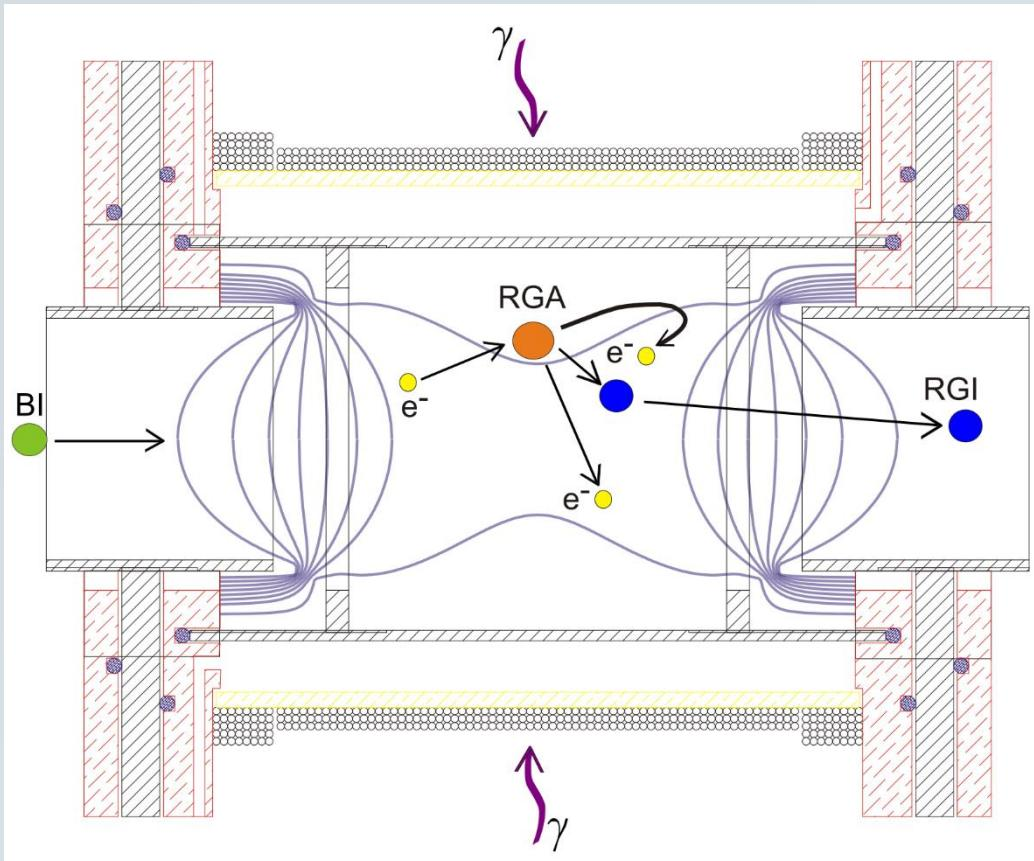
Radial confinement: axial symmetric magnetic field
