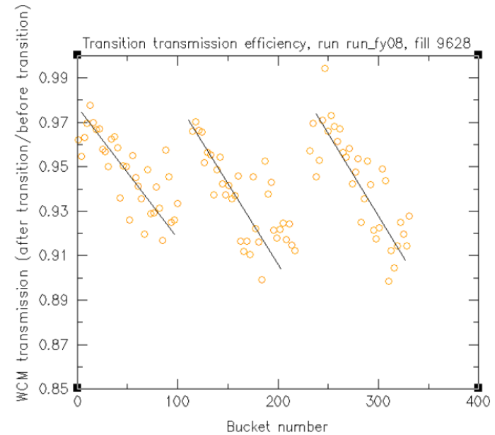
Figure 2: Bunch intensity transmission through the transition in dependence on bunch position in the train.
