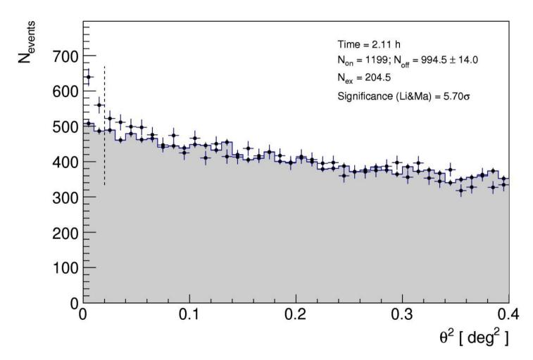
Distribution of the squared angular distance,  $\theta^2$ , between the reconstructed source position and the nominal source position (points) or the background estimation position (shaded area). The vertical dashed line shows the value of  $\theta^2$  up to which the number of excess events and significance are computed.
