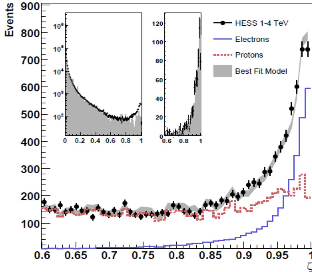
Fig. 1: shows the experimentally measured distribution (black dots) of the zeta parameter compared with the simulated distributions of electrons and protons for the reconstructed energy range 1–4 TeV.
