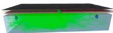
Figure 2: Basic detector station, with one WCD covered with RPCs and a thin slab of lead. The green lines show the tracks of the Cherenkov photons produced by the electron and positron from the conversion of a photon in the lead (for better visualisation the Tyvek's reflectivity was scaled by 1/10).
