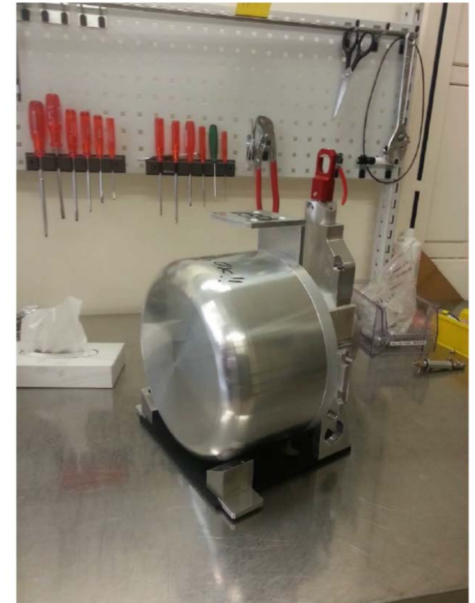
CNMO M11 type container used for the shipment from PSI to CERN
