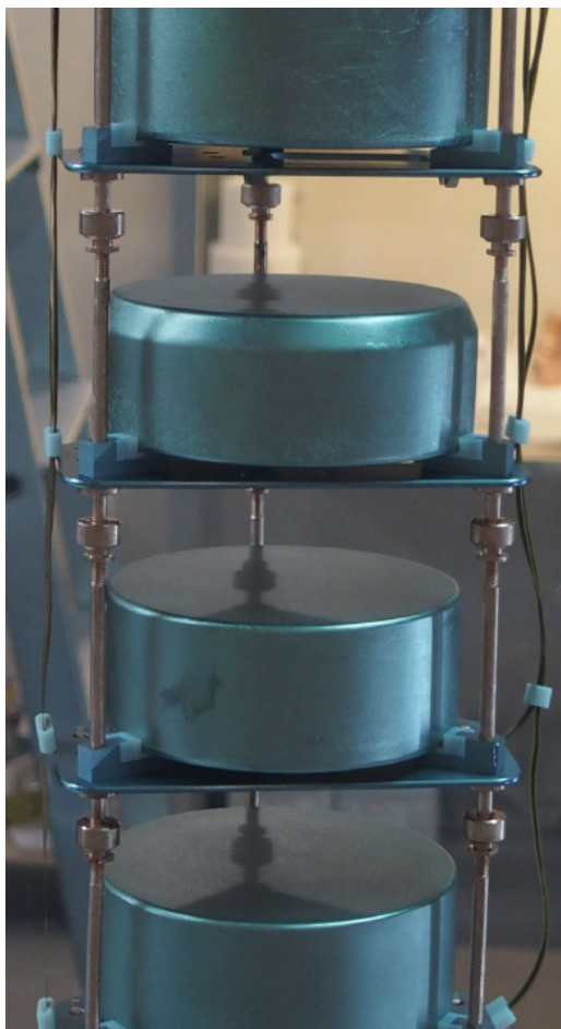
New low-mass detector holder (silicon, copper, PTFE)
