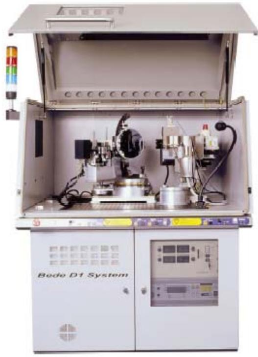
D1 X-ray diffractometer
