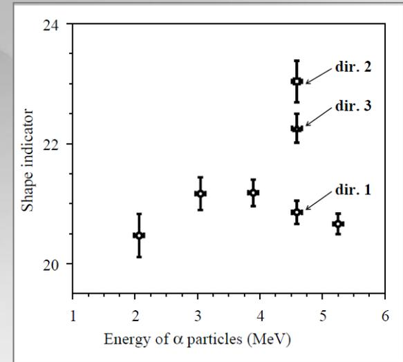
These anisotropic effects are ascribed to preferred directions of the excitons' propagation in the crystal lattice affecting the dynamics of the scintillation mechanism
