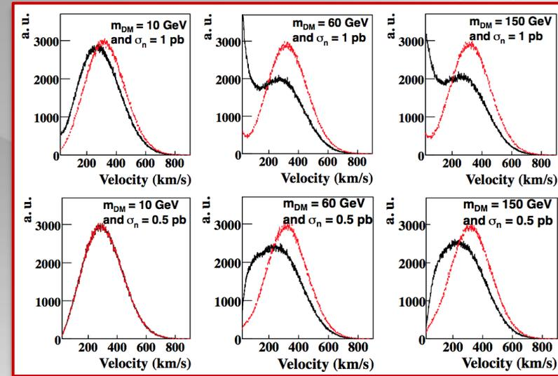
Expected counting rate for a given mass, cross section and scenario by MC:
