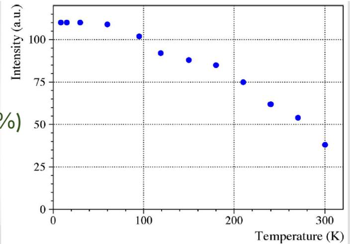
Light output measured for a ZnWO<sub>4</sub> scintillator with  $^{241}\text{Am}$   $\alpha$  particles as function of Temperature
