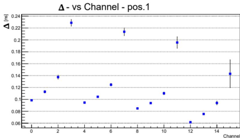
Time difference between the main photon paths from the two fibers, *i.e.*
