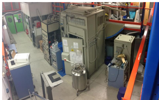
Test facilities (3 dilution fridgew)
