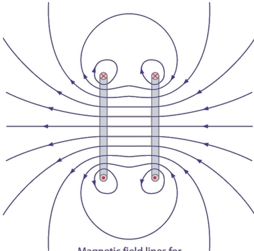
Magnetic field lines for Helmholtz coils.
