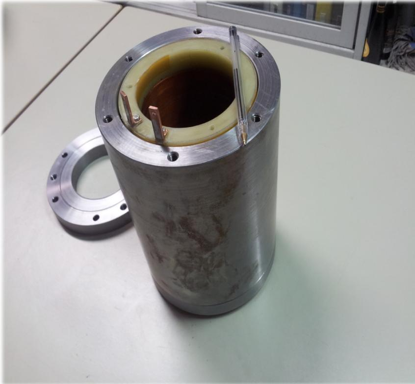
The coil of the primary winding was not designed for the purpose of a good uniformity of the magnetic field because he was designed as pure solenoid with the following radius over length ratio
