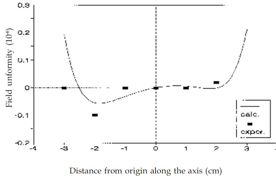
The measured and calculated field uniformity near the center of the 5-current solenoid
