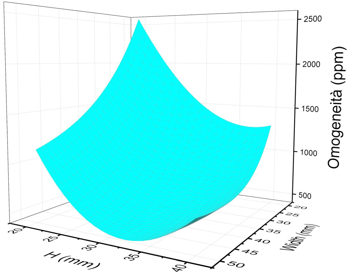
The best inhomogeneity of **411 ppm** is obtained with  $W_{\text{corr}}=50$  and  $H_{\text{corr}}=32$  mm
