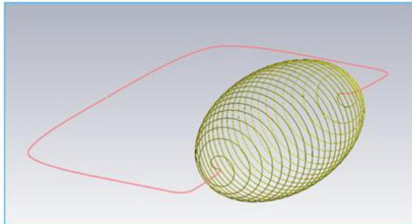
Spheroidal Helical Coil w/ 25 windings of copper wire having 0.9 mm diameter.
