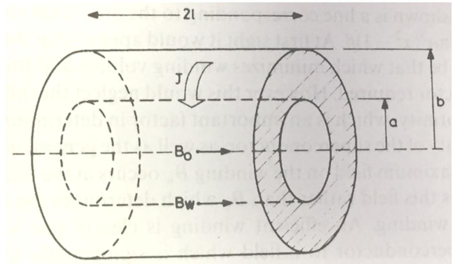
where  $l$  is the coil length while  $a$  and  $b$  are the inner and outer coil radius, respectively
