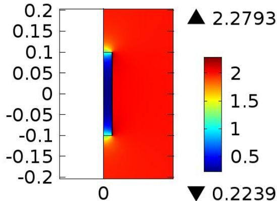
In a cylindric superconducting cavity, even without ending plugs the field inside is fully shielded: FEM with a uniform field 0->2T and  $J_{c0}=2 \cdot 10^9$  A/m<sup>2</sup> and a “Bottura style”  $J_c(B)$ .
