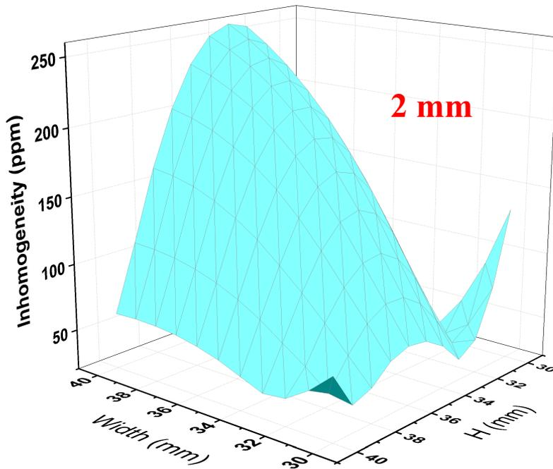
The best inhomogeneity of **31 ppm** is obtained with  $W_{\text{corr}}=33$  and  $H_{\text{corr}}=30$  mm
