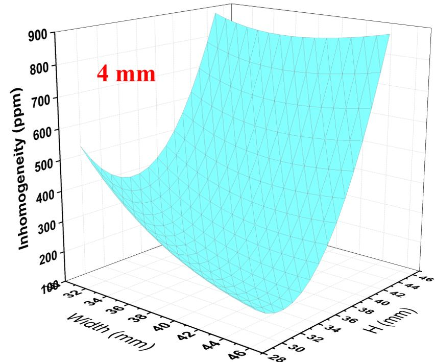
The best inhomogeneity of **132 ppm** is obtained with  $W_{\text{corr}}=45$  mm e  $H_{\text{corr}}=33$  mm
