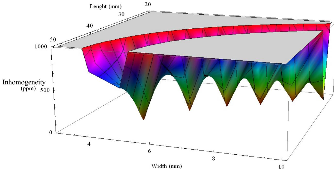
The best homogeneity of **39.5 ppm** is obtained with  $W_{\text{corr}}=5$  and  $H_{\text{corr}}=43$  mm
