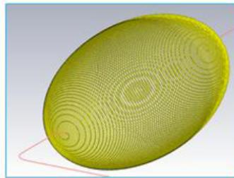
Spheroidal Helical Coil w/ 100 windings of copper wire having 0.9 mm diameter.
