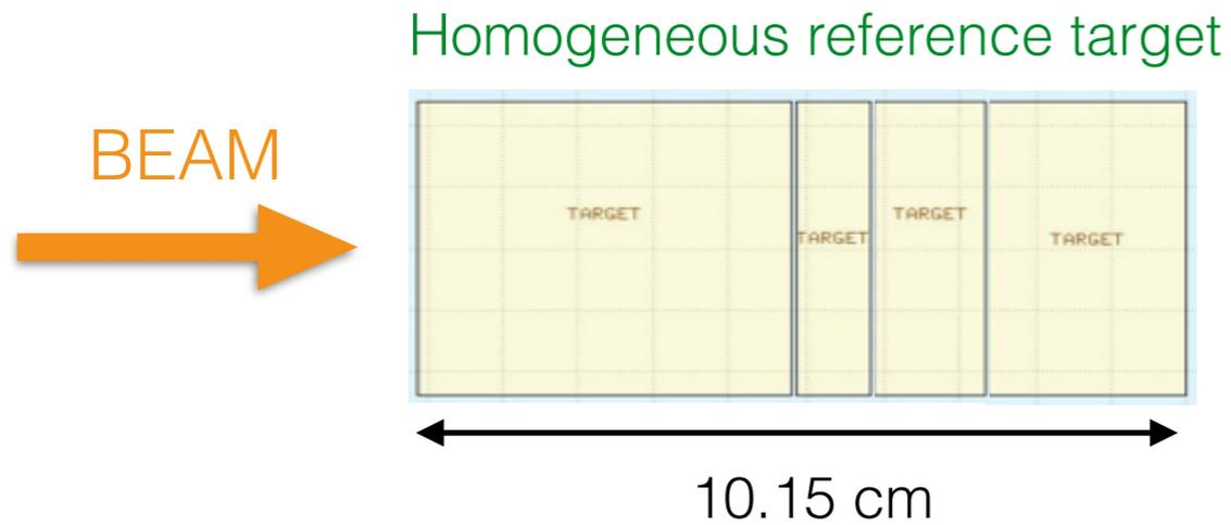
Segmented target, with air gaps
