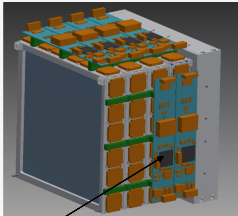
16 FPGA provides the read-out of all ASIC
