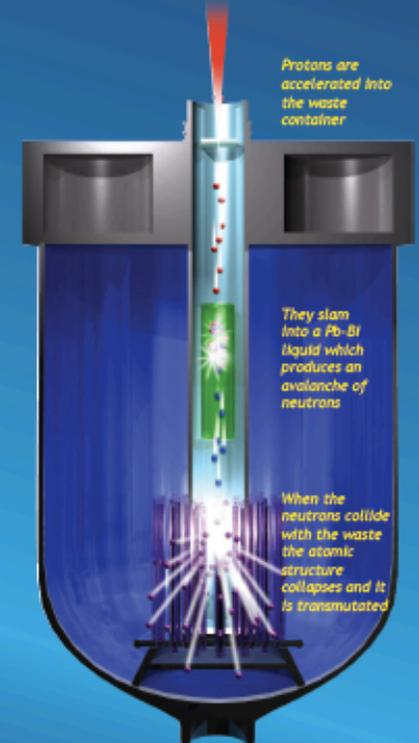
Protons are accelerated into the waste container
