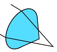
Refractive axicon Pros: Simplest to implement, standard optical component Cons: B-integral, chromatic aberrations, dispersion
