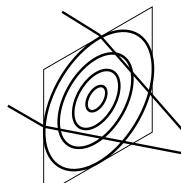
• Diffractive axicon (phase plate) Pros: Less B-integral and dispersion than refractive axicon Cons: non-standard component, chromatic aberrations
