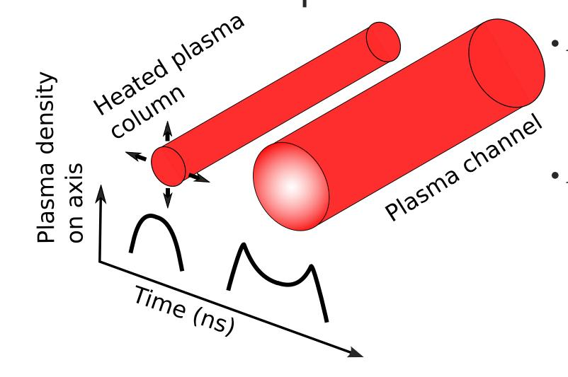
• A heated plasma column with a diameter of 10's of µm is produced at the line focus of an axicon
