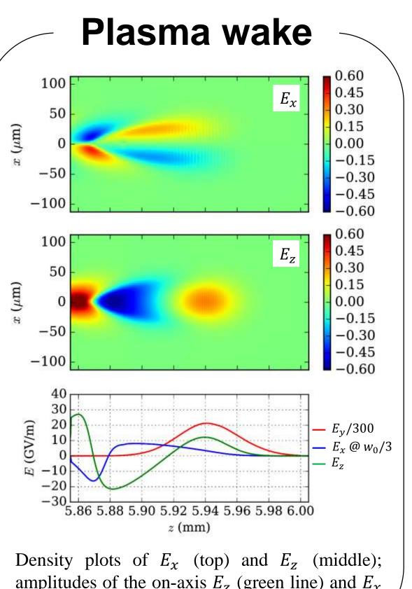
amplitudes of the on-axis  $E_z$  (green line) and  $E_x$ (blue line); channel depth  $\Delta n/\Delta n_c = 0.68$
