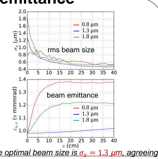
The optimal beam size is  $\sigma_x = 1.3 \ \mu m$ , agreeing well with theories
