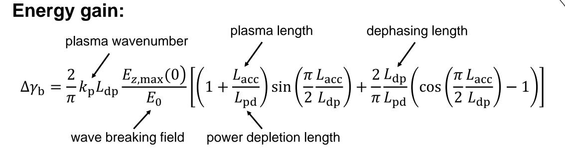
$E_{z,\text{max}}(0) \simeq 0.76 a_0^2 E_0/2\gamma_{\perp}$  is the amplitude of the acc. field (with resonant pulse length)
