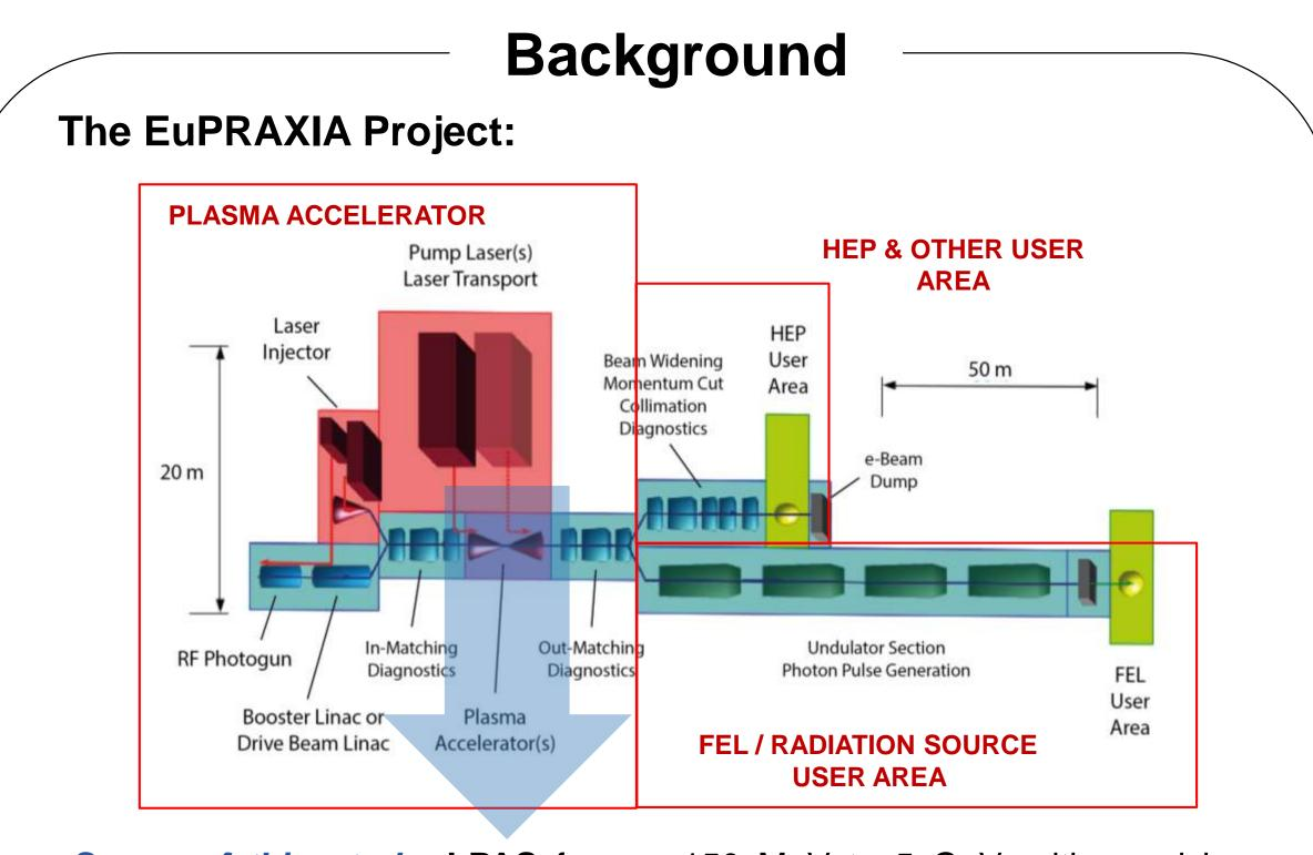
Scope of this study: LPAS from ~ 150 MeV to 5 GeV, with good beam quality, e.g., low emittance and low energy spread, suitable for X-ray FELs
