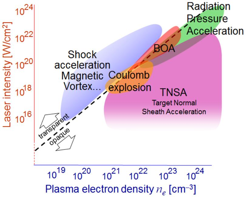
Sheath (surface) acceleration: (in  $\mu\text{m}$ -thick targets)
