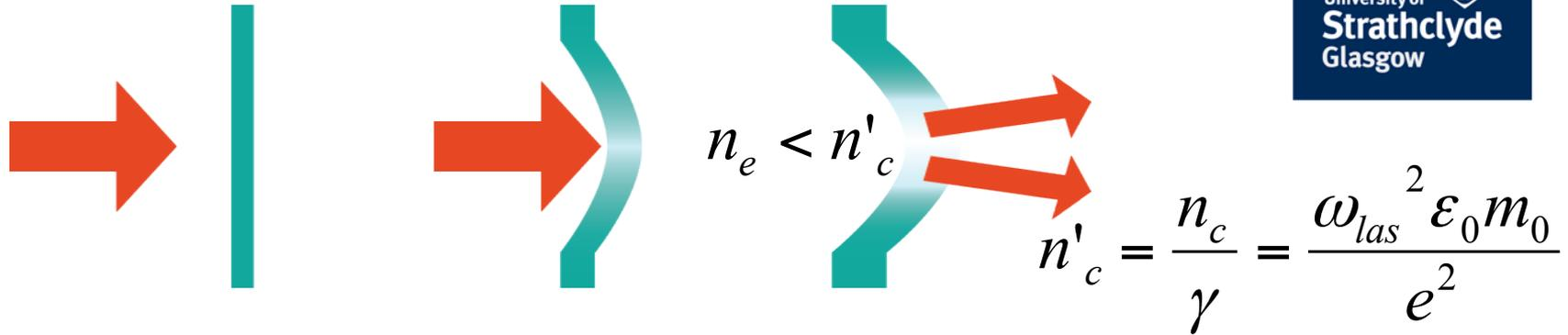
Decrease in relativistic plasma frequency near the peak of the focus produces relativistically induced transparency over a diameter of a few times the laser wavelength
