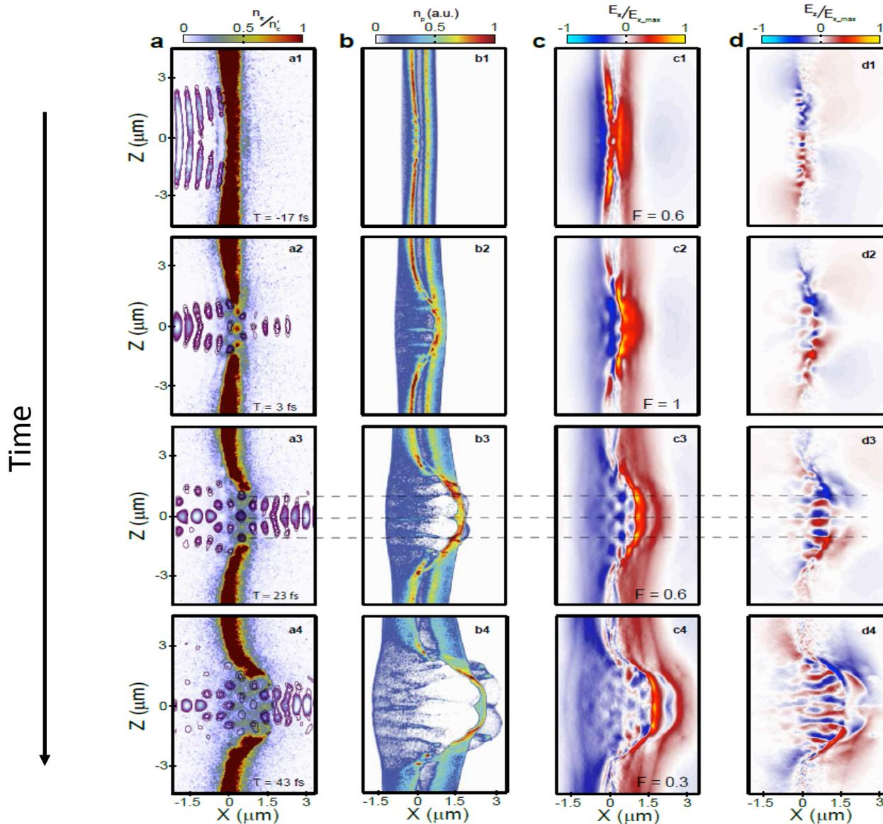
Electron density structure mapped into the proton beam via modulation of the electrostatic field
