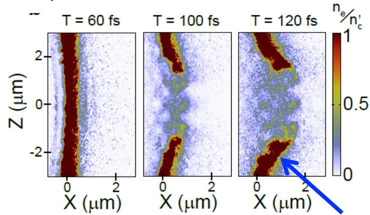
Deformation due to radiation pressure
