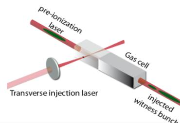
Sharp on-axis plasma density gradients from distinct H<sub>2</sub> and He ionization
