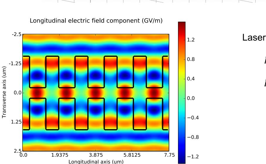
Laser polarization for ACCELERATION:  $\hat{E}_1 = \hat{A}(x,y,z,t)^* \sin(\omega_0 t + \varphi_{01})$   $\hat{E}_2 = \hat{A}(x,y,z,t)^* \sin(\omega_0 t + \varphi_{02})$   $\hat{A}(x,y,z,t) = \begin{pmatrix} A(x,y,z,t) \\ 0 \\ 0 \end{pmatrix}$   $\varphi_{01} = \varphi_{02}$
