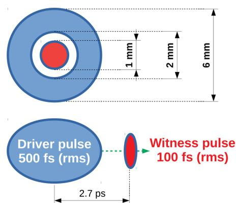
Laser setup on the photo-cathode. The driver pulse has a donut-shape transverse profile, with its hole larger than the dimensions of the witness pulse. The temporal order of the pulses is reversed with respect to the final bunch configuration since it will be rotated and longitudinally compressed during VB. Since space-charge forces would push the particles toward the axis of the hollow driver, its transverse size is set in order to avoid it.
