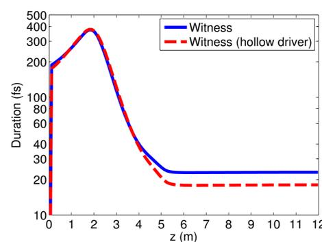
For these reasons we employed a donut-like transverse profile for the driver. We use a hollow driver laser pulse on the photo-cathode and tune the magnetic optics of the photo-injector in order to preserve such a profile during the bunch crossing. The witness thus undergoes its own compression, down to 18 fs (−21%) without being affected by the driver space-charge effects ( $0.9 \mu\text{m}$  emittance, i.e. −35%).
