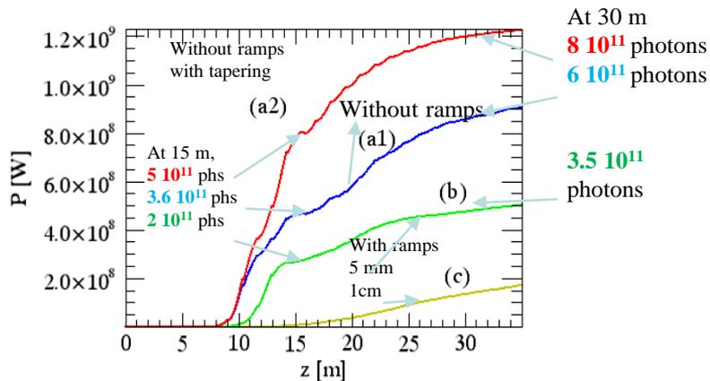
FEL Genesis simulation with **particle driven plasma accelerated electron beams (WP1)**
