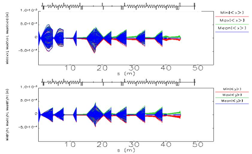
**WP1** results: Centroid distribution at the capillary entrance (above) and trajectory envelope (right) for  $70\mu\text{m}$  misalignment on RF and magnetic elements,  $150\mu\text{m}$  girder to girder, and 0.1% jitter on quadrupole strength and steerer kick after trajectory correction.
