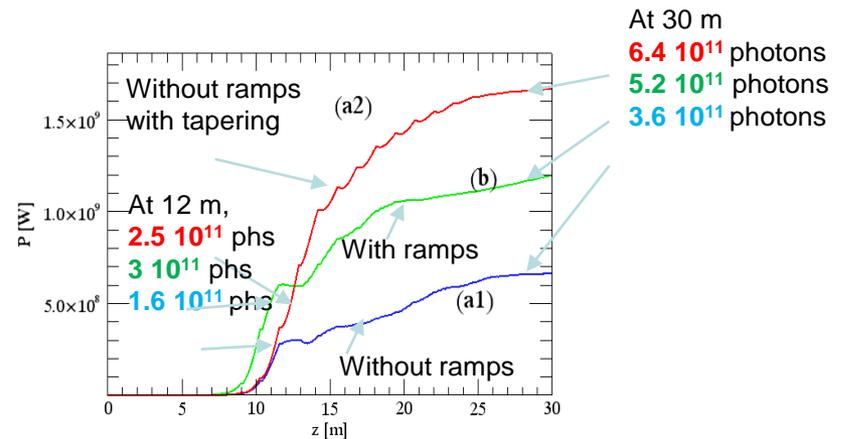
FEL Genesis simulation with **laser driven plasma accelerated electron beams (WP1)**
