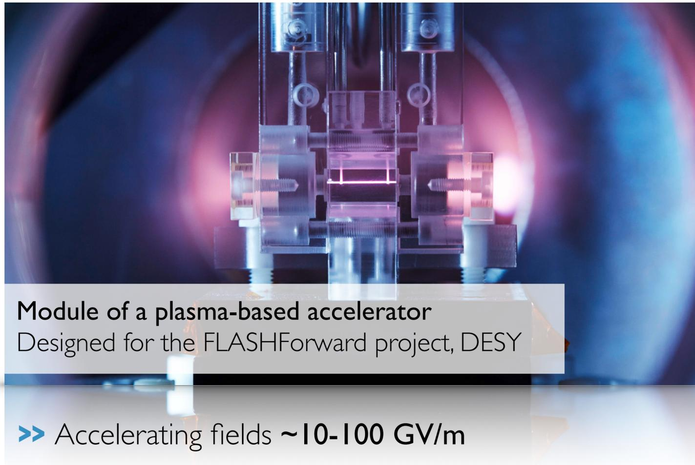
**Module of a plasma-based accelerator**
