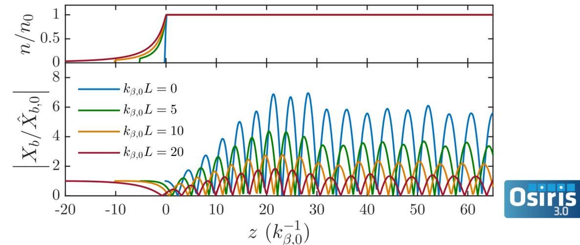
Density profiles and centroid oscillations for different  $\lambda$
