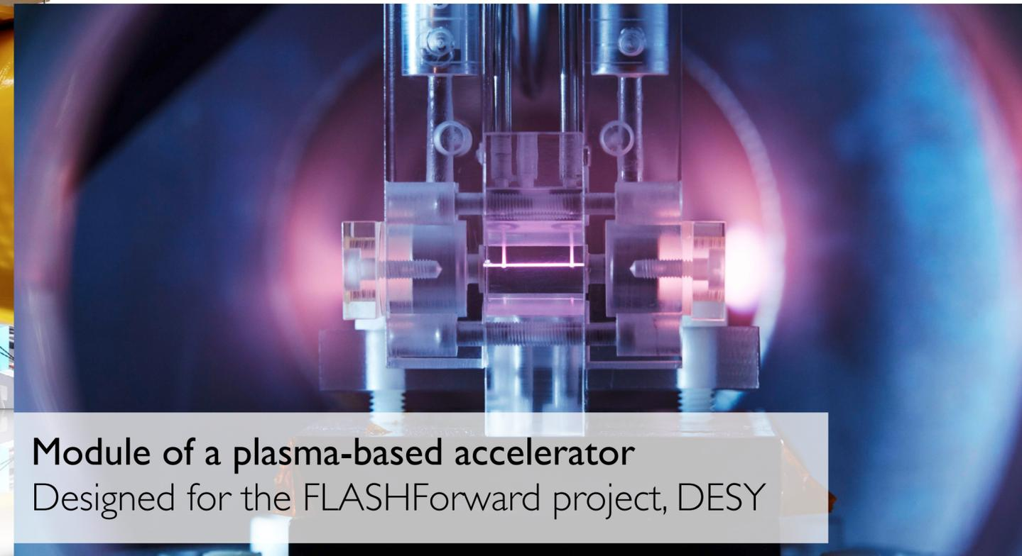
Module of a plasma-based accelerator
