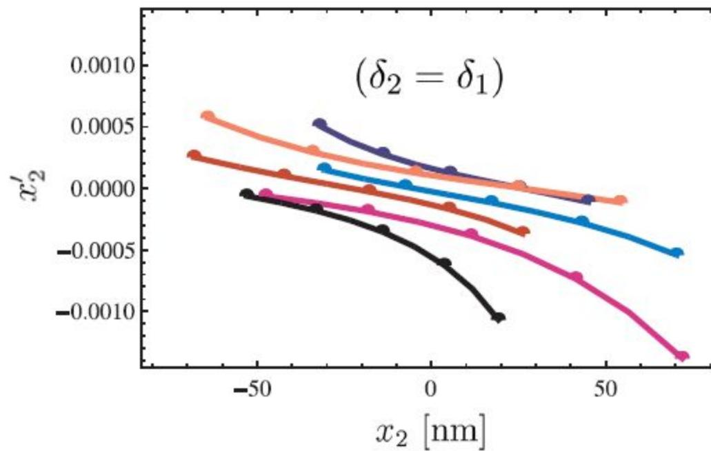
FIG. 10. The focusing properties of the  $\mathcal{O}_{5+1/2}\mathcal{R}^8\mathcal{O}_{5+1/2}\mathcal{R}^8$  segment calculated using “spoiled” ( $\delta_2 = \delta_1$ ) transfer function [compare with the correct result in Fig. 7(c)].
