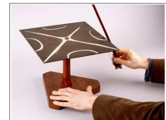
**Image 2** Dr Rees demonstrates the production of a pattern on a Chladni plate using a violin bow.
