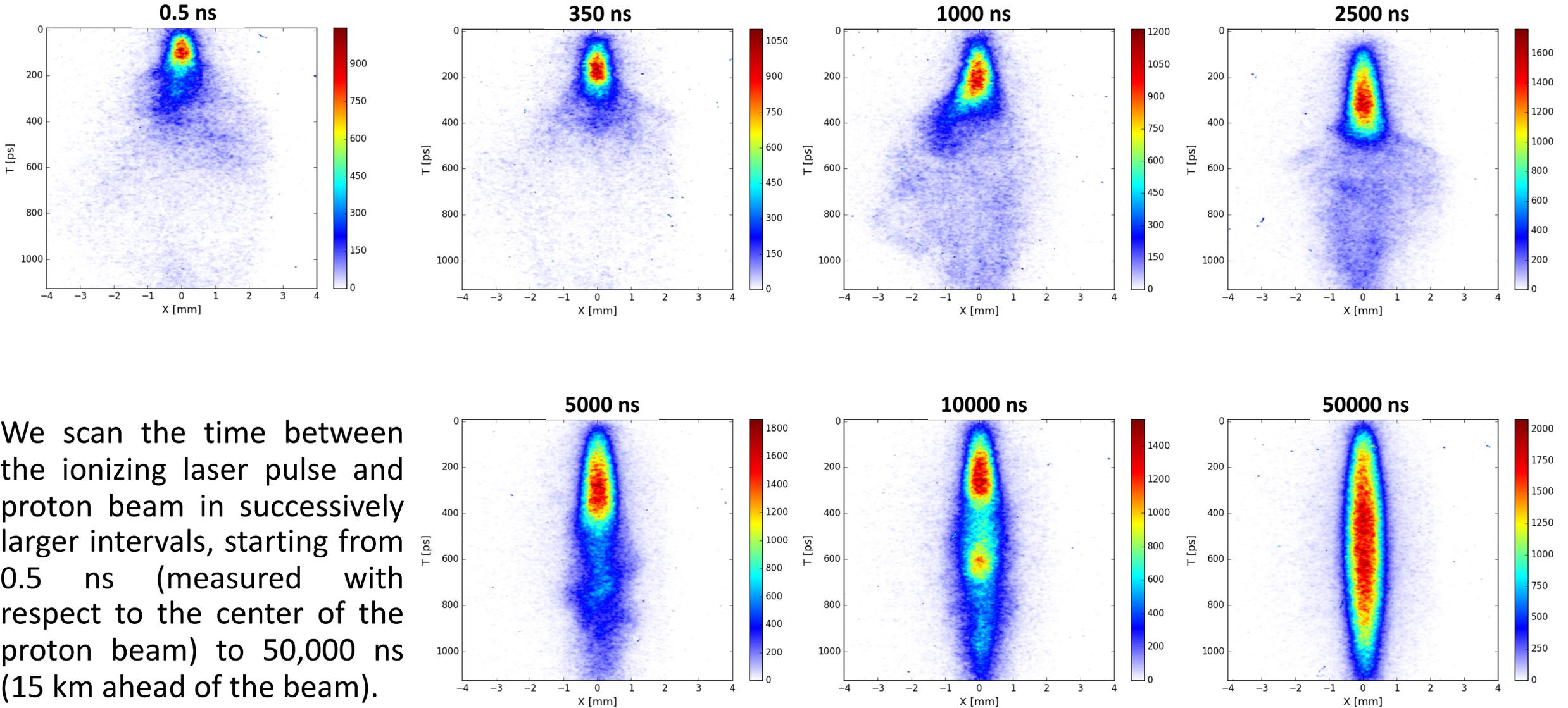
We scan the time between the ionizing laser pulse and proton beam in successively larger intervals, starting from 0.5 ns (measured with respect to the center of the proton beam) to 50,000 ns (15 km ahead of the beam).
