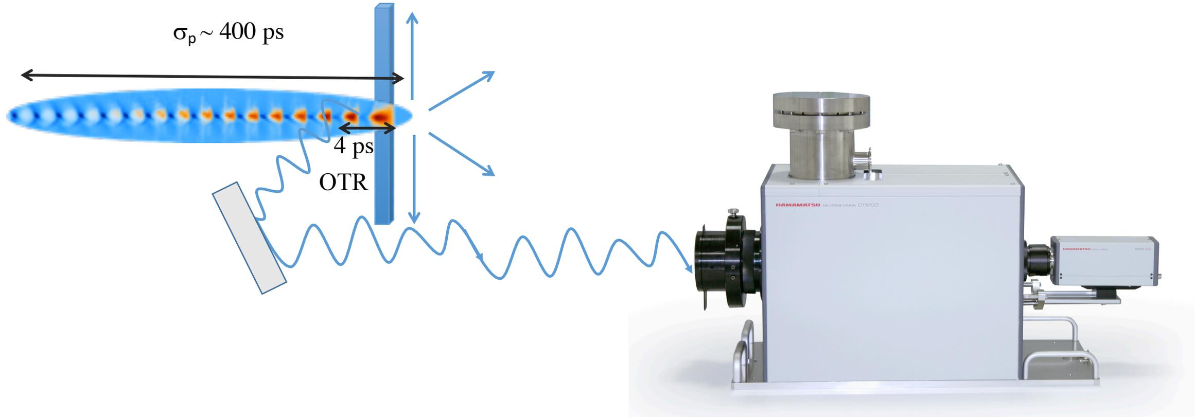
The modulated proton bunch is sent through a metal foil where it generates optical transition radiation (OTR). This radiation is sent to the streak camera.
