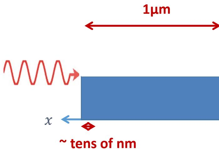
Carbon nanotube foam(CNF): ~1% solid density, highly homogenous at um scale, as thin as a few um, will become homogenous plasma with density around critical density, can be used as plasma optics
