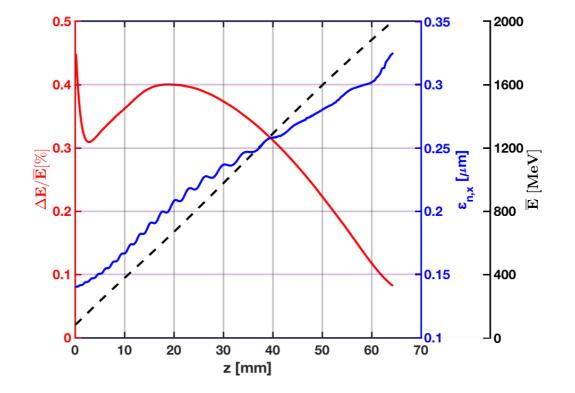
Evolution of the externally injected electron beam properties during acceleration to 2 GeV: relative energy spread (red solid curve); normalized transverse emittance (blue solid curve); mean energy (black dashed curve). Plasma ramp = 0.1 mm. Offset between the electron beam center and the laser pulse center =  $88.3 \mu m$ .
