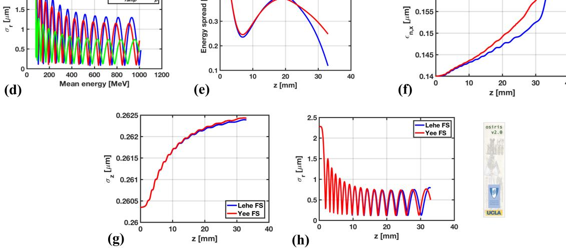
Evolution of the externally injected electron beam properties during acceleration to 1 GeV: normalized transverse emittance (a), relative energy spread (b), longitudinal bunch length (c) and bunch width (d). Plasma ramp = 0.1 mm, 0.74 mm, 5.3 mm. Offset between the electron beam center and the laser pulse center =  $103.25 \mu m$ . Comparison between the Yee and Lehe field solvers (e, f, g, h).
