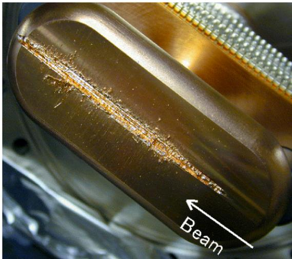
Groove on a movable mask head dug directly by the beam
