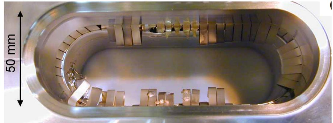
Gasket vacuum leak due to SR
