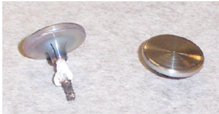
Melted feed-through of a lower button and the fallen upper button (S. Weathersby, ICAP09)
