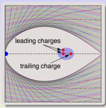
In the absence of theory some researchers<sup>2</sup> use for the *short-range wakefields* formulas that work for a round pipe with resistive wall, corrugated pipe,<sub>z</sub> diefectric pipe, etc. They replace the pipe radius *a* in these formulas by the bubble radius  $r_b$  at the location of the source charge,
