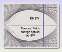
The source charge is now off axis, the offset is assumed small. The shock wave is not axisymmetric,  $E_r \propto \hat{D}(r, \xi) \cos \theta$ ,  $E_{\theta} \propto \hat{D}(r, \xi) \sin \theta$ . Behind the wave  $\Delta E_z(r, \xi, \theta) = \Delta \hat{E}_z(r, \xi) \cos \theta$ . The fields satisfy the following equations
