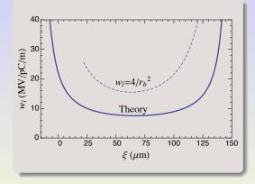
This wake is in good agreement with the simulated jump in  $\Delta E_z$  of a witness charge on the axis of the bubble.
