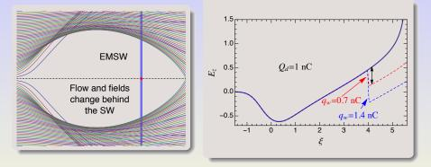
I developed theory that calculates a jump in  $E_z$  immediately behind the witness charge,  $\Delta E_z(r, \xi)$ . Remarkably, the theory predicts that this jump is proportional to the (dimensionless) witness charge  $\nu_w$  (the charge has not to be small). So we can introduce the longitudinal wake is  $w_{\ell} = \Delta E_z(0, \xi)/\nu_w$ .
