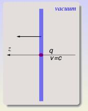
In wakefield theory for relativistic beams we assume v = c. When a point charge q is moving in vacuum, its field is
