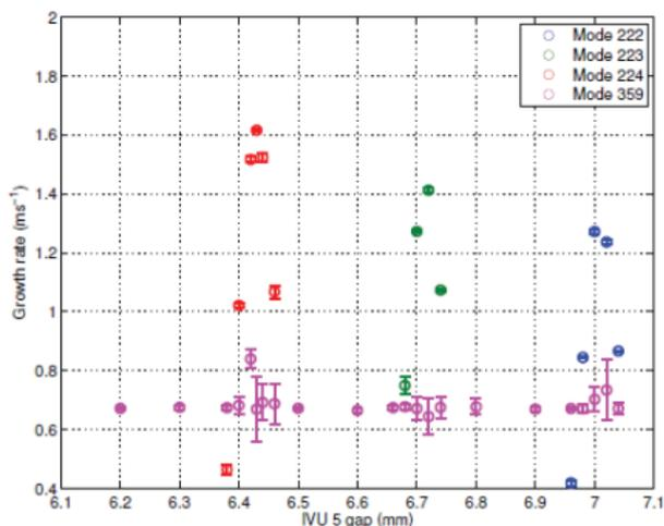
Figure 4: Instability mode growth rates for IVU05 vs gap.
