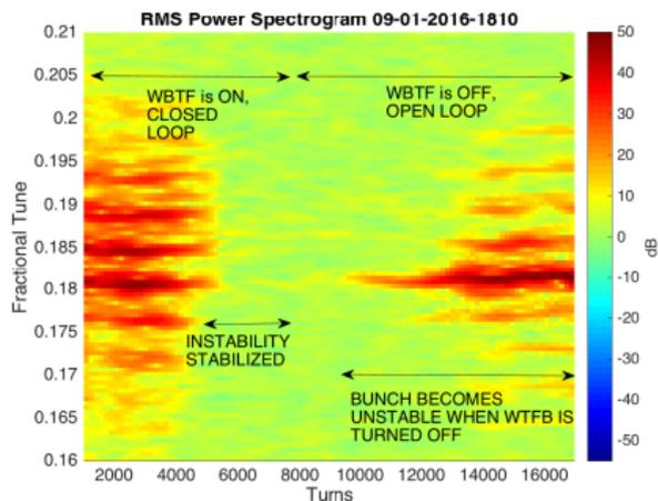
**Figure:** Spectrogram of a bunch. The wideband feedback (WBFB) is ON until turn 8000. The bunch becomes unstable after WBFB is turned OFF.
