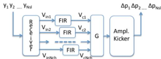
The processing system can be expanded to support more complex off-diagonal (modal) filters, IIR filters, etc as part of the research and technology development
