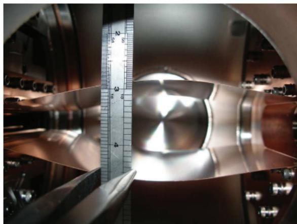
Figure 2: Transition taper view at 6mm gap on IVU5.
