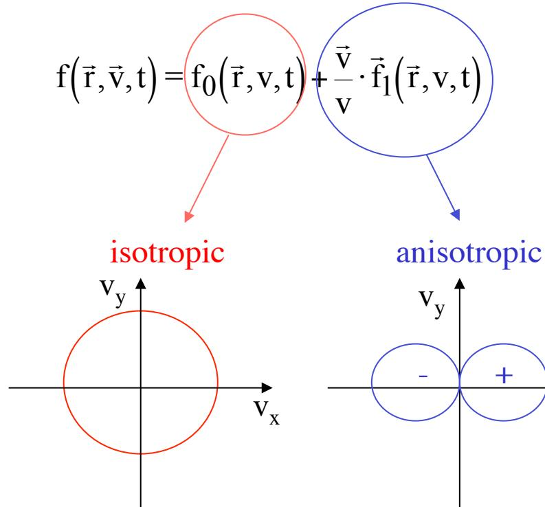
$$\frac{\partial f_0}{\partial t} = -\frac{\partial J_f}{\partial \varepsilon} - \frac{\partial J_{el}}{\partial \varepsilon} - \frac{\partial J_{ee}}{\partial \varepsilon} + S_{in} + S_{sup}$$
