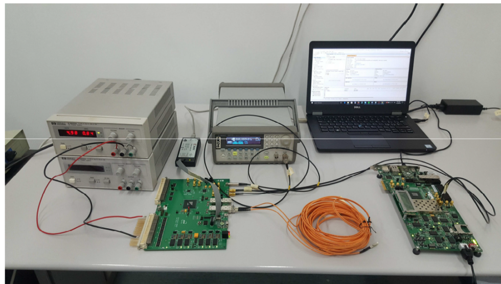
Serial link tested on loopback, with IBERT @ 6.4 Gbps
