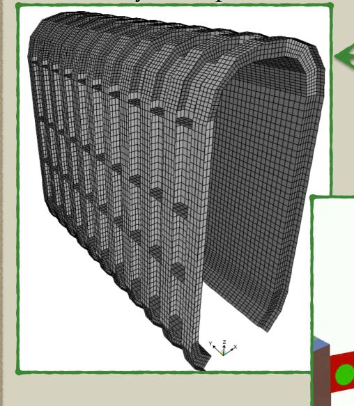
Steel structure with a calendered sheet coupled with welded stiffening elements
