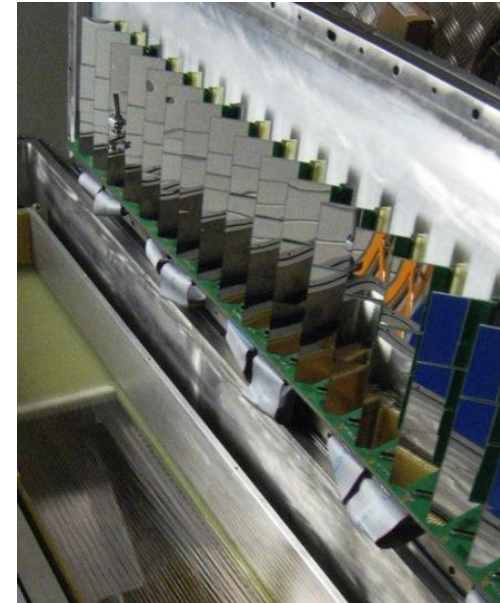
Wall of 60 stopping 7 X 5 cm 2 Silicon detectors Covered area 100 X 20 cm 2 Thickness 500 – 1000 \mu m
