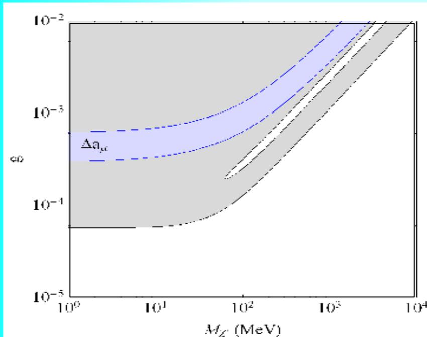
The  $2\sigma$  exclusion region in  $M(Z')$ - $g$ -plane from the COHERENT data. The  $2\sigma$  allowed region that explains the discrepancy in the anomalous magnetic moment of the muon  $\Delta a_\mu = (29 \pm 9) \times 10^{-10}$  is shown for comparison
