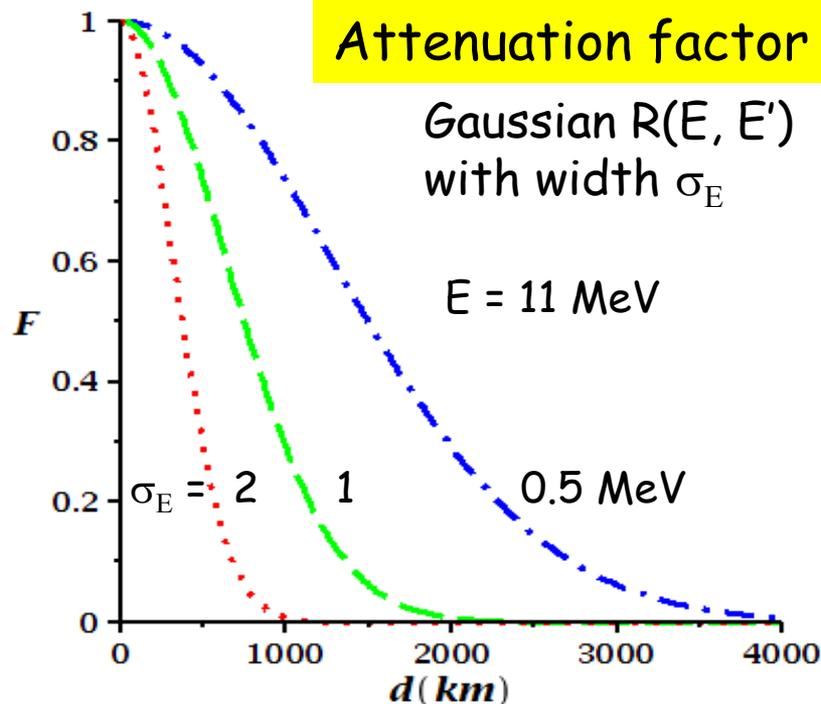
The sensitivity to remote structures  $d > \lambda_{\text{att}}$  is suppressed
