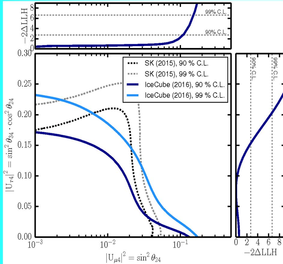
The exclusion limits at 90 % (dark blue) and 99 % C.L. (light blue) using critical values from  $\chi^2$  with 2 d.o.f. The dashed lines show the exclusion from the Super-Kamiokande experiment
