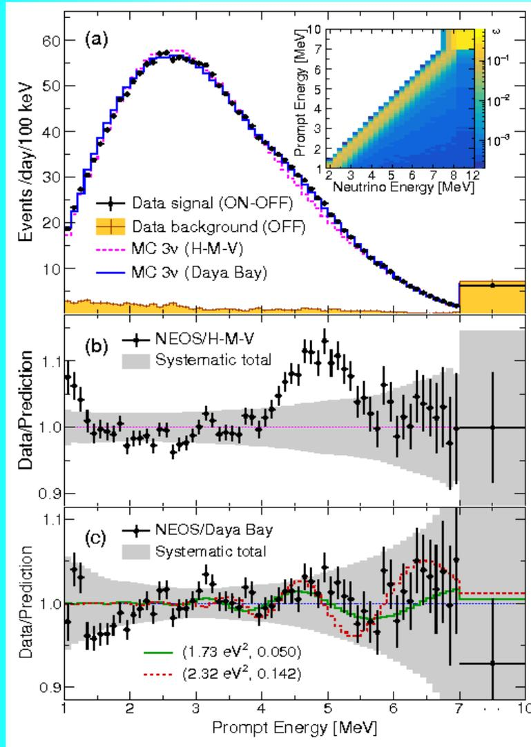
(a) The IBD prompt energy spectrum. The last bin is integrated up to  $10 \sim \text{MeV}$ . The orange shaded histogram is the background (reactor-off)
