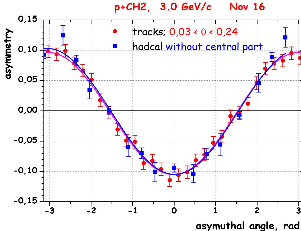
The asymmetry as a function of the azimuthal angle from the calorimeter (blue squares) and from the drift chambers (red circles)
