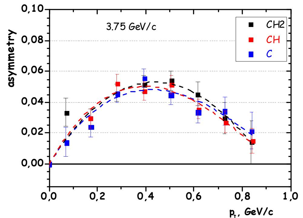
Energy dependence of the neutron asymmetry on CH<sub>2</sub> target.
