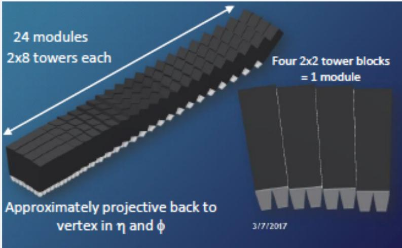
Tungsten-scintillating fiber sampling EMCAL:
