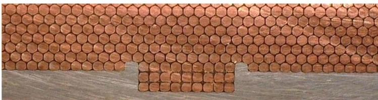
High precision winding technique to guarantee 'orthozyclic winding'
