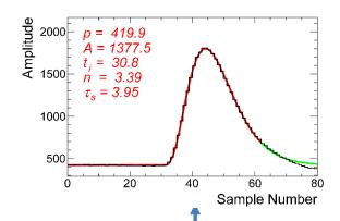
Signal parametrization:  $W(t) = p + A (t - t_i)^n \exp\left(-\frac{t - t_i}{\tau_s}\right)$
