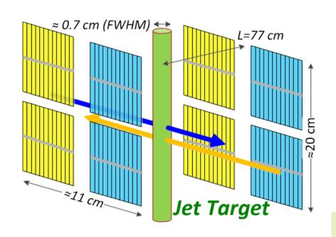
Both RHIC beams (**Blue** and **Yellow**) are measured simultaneously
