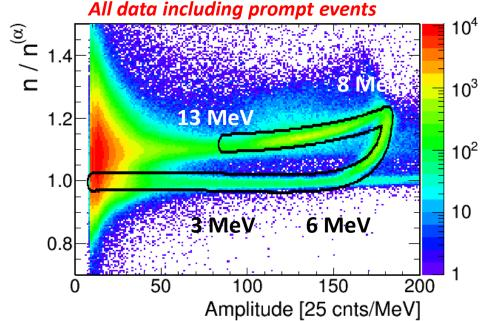
Protons with energy above 7.8 MeV punch through the Si detector. Only part of protons kinetic energy is deposited.
