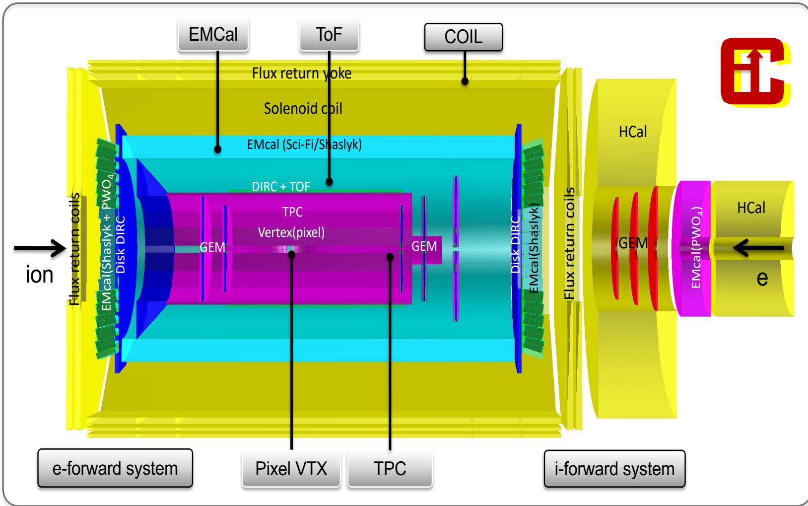
EicC detector systems design and simulation in early stage 22
