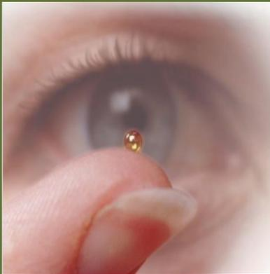
Polarized fuel can be delivered to the plasma using hollow polymer shells (~2 mm diameter ICF pellets)
